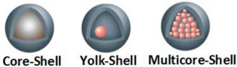
Figure 1.2 Schematic illustration of core–shell, hollow, and yolk–shell catalysts. Adapted with permission from Royal Society of Chemistry (from ref. 5) 5 .
